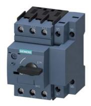
Circuit breaker size S00 for motor protection, CLASS 10 with overload relay function A-release 1.4...2 A N-release 26 A screw terminal Standard switching capacity
