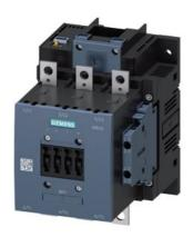
Power contactor, AC-3 185 A, 90 kW / 400 V AC (50-60 Hz) / DC operation 200-277 V UC Auxiliary contacts 2 NO + 2 NC 3-pole, Size S6 Busbar connections Drive: electronic with PLC interface 24 V DC screw terminal
