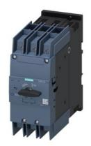
Circuit breaker size S3 for system protection with approval circuit breaker UL 489, CSA C22.2 No.5-02 A-release 30 A N-release 390 A screw terminal
