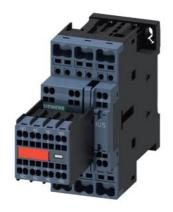
Power contactor, AC-3 17 A, 7.5 kW / 400 V 2 NO + 2 NC, 110 V AC, 50 Hz 120 V, 60 Hz, with inserted varistor, 3-pole, Size S0 Spring type terminal Captive auxiliary switch
