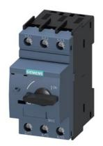
Circuit breaker size S0 for starter combination Rated current 6.3 A N-release 82 A screw terminal Standard switching capacity
