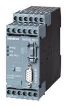
SIPLUS SIMOCODE pro V Basic unit 2 -25...+60°C with conformal coating based on 3UF7010-1AU00-0 . E- type with "Safety ""12 Mbit/s, RS485;""" "4I/3O freely parameterizable;" "US: 110-240V AC/DC; input for" "thermistor connection;" "monostable relay outputs;" expandable by extension modules
