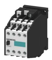
Contactor relay, 62E, DIN EN 50011, 6 NO + 2 NC, screw terminal AC operation 24 V AC 50/60 Hz
