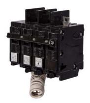
Siemens Low Voltage Molded Case Circuit Breakers General Purpose MCCBs are Circuit Protection Molded Case Circuit Breakers. 3-Pole Common-Trip circuit breaker type BQ. Rated 240 V (060A) (AIR 10 kA). Special features: 120VAC Shunt Trip. Note: Load side lugs are included.
