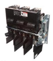
Siemens Low Voltage Circuit Protection OEM Disconnect & Accessories. Type: OEM DISCONNECT SWITCH Std: UL V. Rating: 600V A. Rating: 100A F. Rating: 60Hz Action: SINGLE THROW Enclosure: TYPE 1/3R/12 Mounting: FLANGE MOUNTING Insulation: YES O. Cycles: 10000 O. Temperature: (-20F-120F) AMBIENT TEMPERATURE Environmental Conditions: INDUSTRIAL/OUTDOOR
