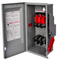
Siemens Low Voltage Circuit Protection Heavy Duty Safety Switches. Type: ENCLOSED, SAFETY SWITCH Std: UL V. Rating: 600V A. Rating: 800A Wattage: 3W No. Of Poles: 3P F. Rating: 60Hz Action: SINGLE THROW Material: 304SS Enclosure: TYPE 3R. 2-3 point mounting holes. O. Cycles: 3500 O. Temperature: (-20F-120F) AMBIENT TEMPERATURE Environmental Conditions: OUTDOOR
