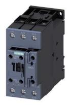
power contactor, AC-3 50 A, 22 kW / 400 V 1 NO + 1 NC, 220 V AC, 50 Hz / 240 V, 60 Hz, 3-pole, Size S2, screw terminal
