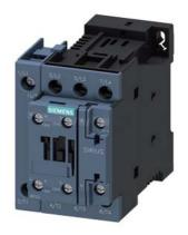
Contactor, AC-1, 35 A/400 V/40  $^{\circ}\text{C}$  , S0, 4-pole, 24 V DC, 1 NO+1 NC, screw terminal
