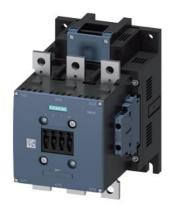
Power contactor, AC-3 265 A, 132 kW / 400 V AC (50-60 Hz) / DC operation 220-240 V UC Auxiliary contacts 2 NO + 2 NC 3-pole, Size S10 Busbar connections Drive: conventional screw terminal
