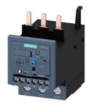
Overload relay 12.5...50 A Electronic For motor protection Size S2, Class 20E Contactor mounting Main circuit: Screw Auxiliary circuit: Screw Manual-Automatic-Reset
