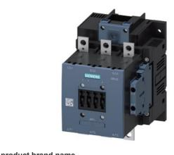
Power contactor, AC-3 185 A, 90 kW / 400 V AC (50-60 Hz) / DC operation 200-220 V UC Auxiliary contacts 2 NO + 2 NC 3-pole, Size S6 Busbar connections Drive: conventional screw terminal
