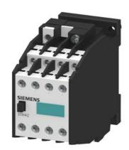
Contactor relay, 80E, DIN EN 50011, 8 NO, screw terminal AC operation 120 V AC 60 Hz/110 V AC 50 Hz
