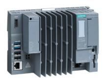
SIMATIC ET 200SP Open Controller, CPU 1515SP PC2 T, 8 GB RAM, 128 GB CFast with Windows 10 IoT Enterprise 64-bit and S7-1500 Software Controller CPU 1505SP T pre-installed, Interfaces: 1x Slot CFast, 1x slot SD/MMC, 1x connection for ET 200SP bus Adapter PROFINET, 1x 10/100/1000 Mbit/s Ethernet, 2x USB 3.0, 2x USB 2.0, 1x display port, Documentation on CFast Restore image on CFast
