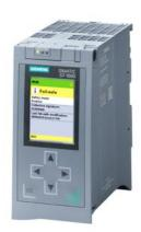
SIMATIC S7-1500T, CPU 1515TF-2 PN, Central processing unit with work memory 750 KB for program and 3 MB for data, 1st interface: PROFINET IRT with 2-port switch, 2nd interface, Ethernet, 30 ns bit performance, SIMATIC Memory Card required
