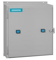
Duplex starter W/O alternator, Size 3, Three phase full voltage, Amb compensate bimetal OLrelay Contactor amp rating 90Amp 110V 50HZ / 120V 60HZ coil, Non-combination type, Enclosure NEMA type 1, Indoor general purpose use
