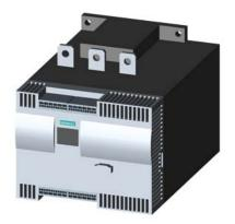
SIRIUS soft starter Values at 460 V, 50 °C standard: 215 A, 150 hp Inside-delta: 372 A, 300 hp 200-460 V AC, 115 V AC spring-type terminals !!! Phased-out product !!! Successor is SIRIUS 3RW5, Preferred successor type is >>3RW5544-2HA14<<
