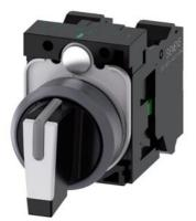
Selector switch, illuminable, 22 mm, round, plastic with metal front ring, white, selector switch, short, 3 switch positions I>O<II, momentary contact type, actuating angle 2x45°, 10:30h/12h/13:30h, with holder, 1 NO, 1 NO, spring-type terminal, with laser labeling, upper case and lower case, always upper case at beginning of line
