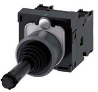
Coordinate switch, 22 mm, round, plastic with metal front ring, black, 2 switch positions, vertical latching, with mechanical interlocking, in O position, with holder, 1 NO, 1 NO, screw terminal, with laser labeling, lower case
