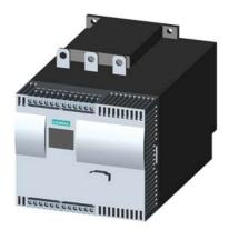
SIRIUS soft starter Values at 575 V, 50 °C standard: 145 A, 125 hp Inside-delta: 251 A, 250 hp 400-600 V AC, 115 V AC spring-type terminals !!! Phased-out product !!! Successor is SIRIUS 3RW5, Preferred successor type is >>3RW5536-2HA16<<
