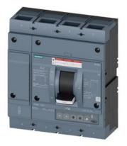
circuit breaker 3VA6 UL frame 1000 breaking capacity class C 100kA @ 480 V 4-pole, line protection ETU330, LIG, ln=1000A overload protection lr=400A ...1000A short circuit protection li=1,5...10 x ln
