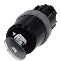
key-operated switch Siemens, 22 mm, round, plastic with metal front ring, lock number SSG10, with 2 keys, 2 switch positions O<I, momentary contact type, actuating angle 45°, 10:30h/12h, key removal O, with laser labeling, upper case and lower case, always upper case at the beginning of the word
