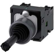
Coordinate switch, 22 mm, round, plastic with metal front ring, black, 2 switch positions, horizontal latching, without mechanical interlocking, in O position, with holder, 1 NO, 1 NO, screw terminal, with laser labeling, lower case
