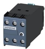
solid-state time-delayed front-side auxiliary switch Time range 5...100 s, 200 ... 240 V AC, 1 NO contact, 1 NC contact ON delay, for 3RT1
