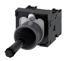
Coordinate switch, 22 mm, round, plastic with metal front ring, black, 2 switch positions, vertical latching, with mechanical interlocking, in O position, with holder, 1 NO, 1 NO, screw terminal, with laser labeling, upper case
