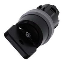
Key-operated switch O.M.R, 22 mm, round, plastic with metal front ring, lock number 73034, black, with 2 keys, 2 switch positions O-I, latching, actuating angle 90°, 10:30h/13:30h, key removal I, with laser labeling, inscription or symbol Customer-specific selection with SIRIUS ACT configurator (CIN)
