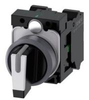
Selector switch, illuminable, 22 mm, round, plastic with metal front ring, white, selector switch, short, 3 switch positions I-O-II, latching, actuating angle  $2x45^{\circ}$ , 10:30h/12h/13:30h, with holder, 1 NO, 1 NO, spring-type terminal, with laser labeling, upper case and lower case, always upper case at the beginning of the word
