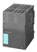
Communications processor CP 343-1 Advanced for connection of SIMATIC S7-300 CPU to Industrial Ethernet: PROFINET IO controller a./o. IO device; RT and IRT, MRP, PROFINET CBA; TCP/IP, ISO, UDP, S7 comm., S5-compat. communication (SEND/RECEIVE) with Fetch/Write RFC1006, Multicast Diagnostic extension, SNMP, DHCP, FTP client/server, e-mail, Gigabit-SS1X RJ45 (10/100/1000) PROFINET interface 2x RJ45 (10/100 Mbit); PROFINET CBA; security (firewall/VPN); PROFIenergy
