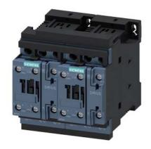
Reversing contactor assembly AC-3, 7.5 kW/400 V, 24 V DC 3-pole, Size S0 screw terminal electrical and mechanical Interlock 2 NO integrated
