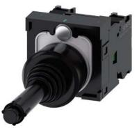
Coordinate switch, 22 mm, round, plastic, black, 2 switch positions, vertical, momentary contact type, with mechanical interlocking in O position, with holder, 1 NO, 1 NO, screw terminal, with laser labeling, upper case and lower case, always upper case at beginning of line
