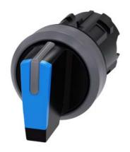
Selector switch, illuminable, 22 mm, round, plastic with metal front ring, blue, selector switch, short, 3 switch positions I-O<II, left latching, right momentary contact type, actuating angle 2x45°, 10:30h/12h/13:30h, with laser labeling, inscription or symbol Customer-specific selection with SIRIUS ACT configurator (CIN)
