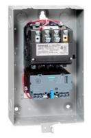
Non-reversing motor starter Size 1 Three phase full voltage Solid-state overload relay OLRelay amp range 10-40a 190-220/220-240V 50/60HZ coil Combination type Indoor general purpose use
