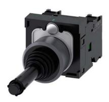
Coordinate switch, 22 mm, round, plastic with metal front ring, black, 2 switch positions, horizontal, momentary contact type, with mechanical interlocking in O position, with holder, 1 NO, 1 NO, screw terminal, with laser labeling, upper case and lower case, always upper case at beginning of line
