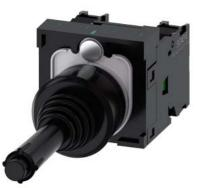
Coordinate switch, 22 mm, round, plastic, black, 2 switch positions, vertical latching, with mechanical interlocking, in O position, with holder, 1 NO, 1 NO, screw terminal, with laser labeling, upper case
