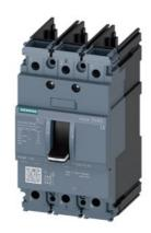
circuit breaker 3VA5 UL frame 125 breaking capacity class S 25kA @ 480V 3-pole, line protection TM210, FTFM, In=15A overload protection Ir=15A fixed short-circuit protection Ii=20 x In UL 489 SB (naval), 50° C without connection
