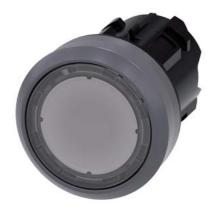
Illuminated pushbutton, 22 mm, round, plastic with metal front ring, clear, pushbutton, flat momentary contact type, with laser labeling, upper case and lower case, Always upper case at the beginning of the word
