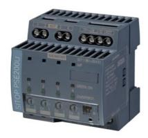
SITOP PSE200U 3 A NEC CLASS 2 Selectivity module 4channel input: DC 24 V/12 A output: 24 V/4x 3A NEC class 2 Level adjustable 0.5-3 A with common signaling contact
