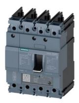
circuit breaker 3VA5 UL frame 125 breaking capacity class M 35kA @ 480 V 4-pole, line protection TM230, FTAM, In=100A overload protection Ir=100A fixed short-circuit protection Ii=5...10 x In N conductor protection 100% without connection
