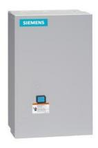
Non-reversing motor starter Size 2 1/2 Three phase full voltage Amb compensate bimetal OLrelay Contactor amp rating 60Amp Non-combination type Enclosure NEMA type 1 Indoor general purpose use Extra-wide enclosure
