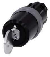
key-operated switch Siemens, 22 mm, round, plastic with metal front ring, special lock, with 2 keys, 3 switch positions I>O<II, momentary contact on the left, latching on the right, actuating angle  $2x45^{\circ}$ , 10:30h/12h/13:30h, key removal II
