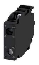
Contact module with 2 contact elements, 1 NO leading + 1 NC lagging, gold-plated contacts, screw terminal, for front plate mounting
