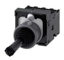
Coordinate switch, 22 mm, round, plastic with metal front ring, black, 4 switch positions, latching, without mechanical interlocking, in O position, with holder, 1 NO, 1 NO, 1 NO, 1 NO, screw terminal, Z=20-unit packaging
