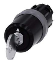
Key-operated switch BKS, 22 mm, round, plastic with metal front ring, lock number S1, with 2 keys, 3 switch positions I-O<II, left latching, right momentary contact type, actuating angle  $2x45^{\circ}$ , 10:30h/12h/13:30h, key removal I, with laser labeling, upper case and lower case,
