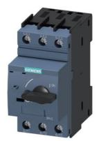
Circuit breaker size S0 for starter combination Rated current 25 A N-release 325 A Screw terminal Standard switching capacity
