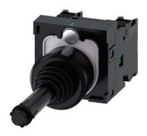
Coordinate switch, 22 mm, round, plastic, black, 2 switch positions, vertical latching, with mechanical interlocking, in O position, with holder, 1 NO, 1 NO, screw terminal, with laser labeling, upper case and lower case, always upper case at beginning of line
