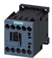
Power contactor, AC-3 16 A, 7.5 kW / 400 V 1 NC, 230 V AC, 50/60 Hz 3-pole, Size S00 screw terminals
