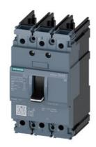
circuit breaker 3VA5 UL frame 125 breaking capacity class S 25kA @ 480V 3-pole, line protection TM210, FTFM, In=40A overload protection Ir=40A fixed short-circuit protection Ii=10 x In UL 489 SB (naval), 50° C without connection
